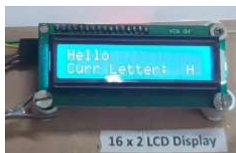
Fig 6.10 :DISPLAYING MESSAGE ON LCD
